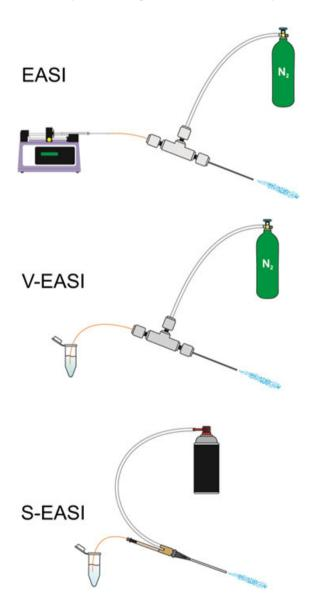
**Figure 2.** The involution of designs (from complex to simple) for EASI sources. EASI simplified the operation of spray-based techniques for ambient desorption/ionization by eliminating voltage and heating. V-EASI further simplified the system by eliminating the need of electrical syringe pumping, whereas S-EASI eliminated the need of cylinders of inert gases (N<sub>2</sub>) using a can of compressed air and very simple, low cost and disposable parts.
