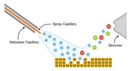
Figure 3. Schematic representation of the EASI mechanism of desorption and ionization. The bipolar stream of minute charged droplets produced by SSI bombard the surface picking up and ionizing the analyte molecules (M) in the form of either positive or negative ions, or both.
