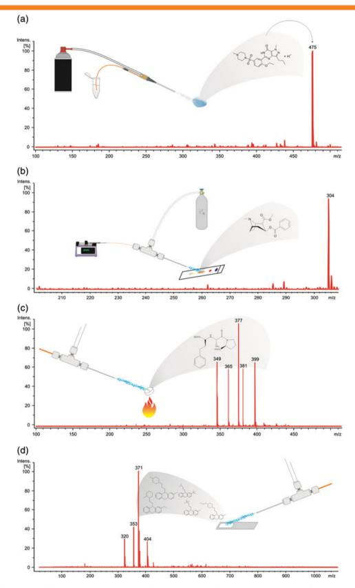
**Figure 4.** Set of applications of fingerprinting EASI-MS (or one of its sister techniques) for (a) the 'sample preparation free' analysis of drugs (sildenafil), (b) the characterization of the cocaine spot in a TLC plate, (c) the direct degradation monitoring of enalapril maleate, and (d) in combination with selective sequesters based on molecularly imprinted polymers (MIP) for the analysis of phenothiazines in urine.
